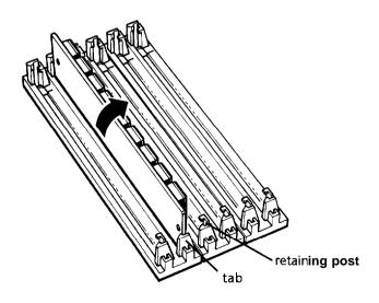
The SIMM should snap into place between the tabs and the retaining posts. If it does not go in smoothly, do not force it; pull it all the way out and try again.
